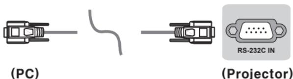
Figure 1: RS-232 Connection Diagram
