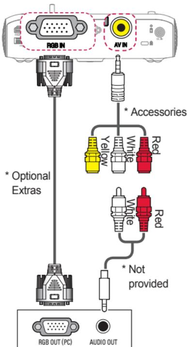
You can connect the audio cable without using a gender as shown in the illustration above.
