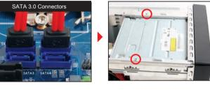
5. Connect the Serial ATA and power cables to the HDD.
