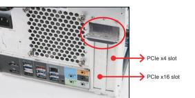
2. Install the PCle x4 / PCle x16 card into the PCle x4 / PCle x16 slots.
