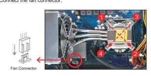
11. Fasten the Smart Fan to the chassis with the four thumbscrews.
