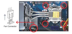
3. Remove the ICE module from the chassis and put it aside.
