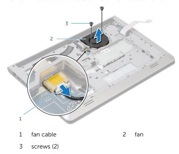
Lift the fan off the base frame.
