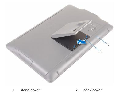
3 Close the stand and remove the screws that secure the stand to the back cover.
