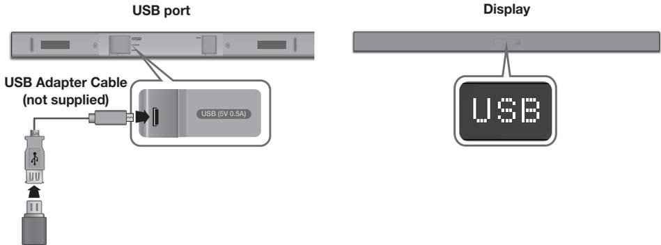
1. Connect a USB adapter cable with a male USB 2.0 Micro USB plug (Type B) on one end and a standard female 2.0 USB jack (Type A) on the other end to the micro USB jack on your Soundbar.
