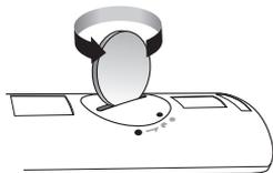
1. Use a suitable coin to turn the remote control's battery cover counterclockwise to remove it as shown in the figure above.
