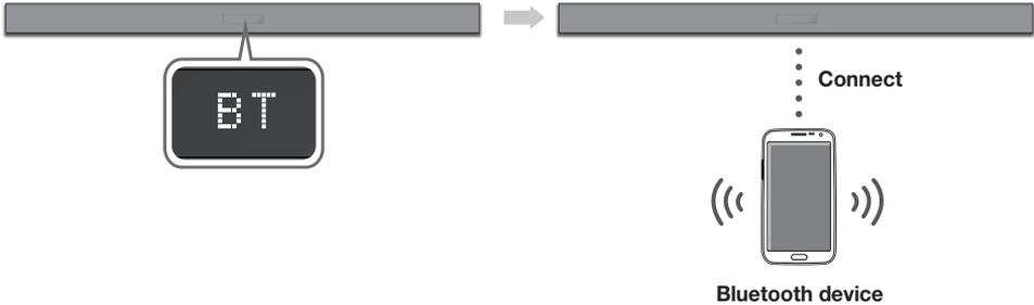
1. Press the
