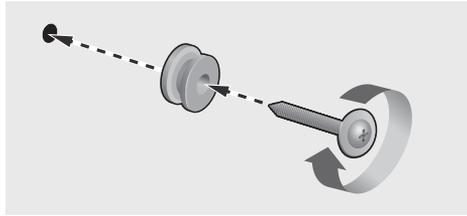
5. Push a screw (not supplied) through each **Holder-Screw**, and then screw each screw firmly into a support screw hole.
