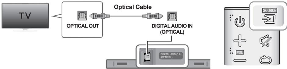
1. Connect the **DIGITAL AUDIO IN** (Audio) jack on the Soundbar to the **OPTICAL OUT** jack of the TV with a digital optical cable.
