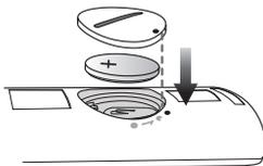
2. Insert a 3V lithium battery. Keep the positive (+) pole facing up when inserting the battery. Put the battery cover on and align the '•' marks side by side as shown in the figure above.
