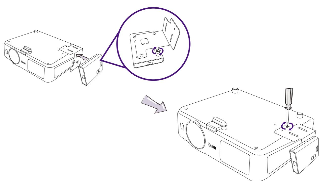
**EN** The new mounting holder helps to fix the wireless receiver to specific BenQ projectors. Depending on the purchased projector model, the wireless receiver may be attached to the right or left side of projector. Refer to the following illustrations and the model list for the appropriate location and the installation procedures. Place the projector bottom up before you start the installation.
