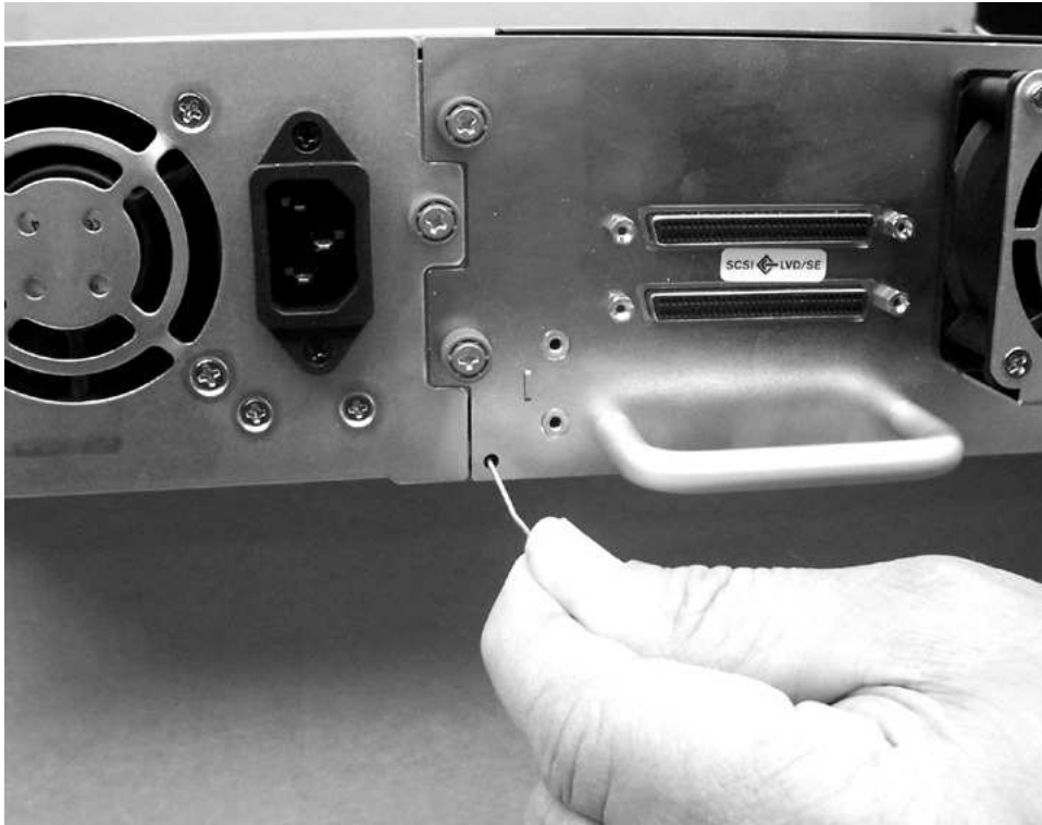
Figure 132. Access holes for the left magazine
