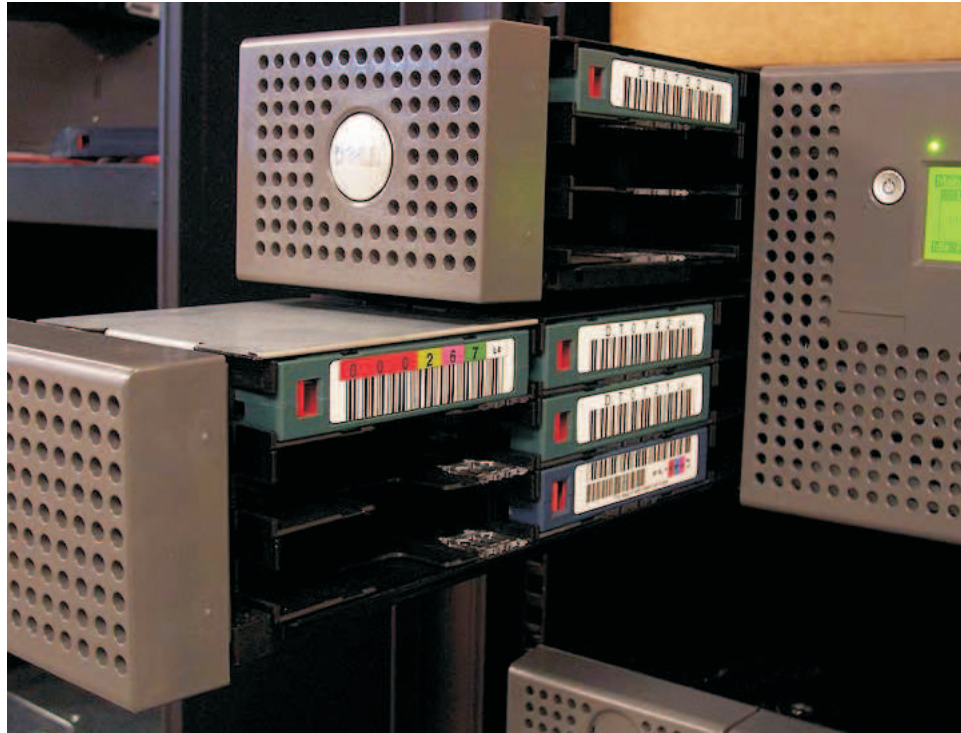
Figure 62. 4U library I/O station in the lower left magazine
