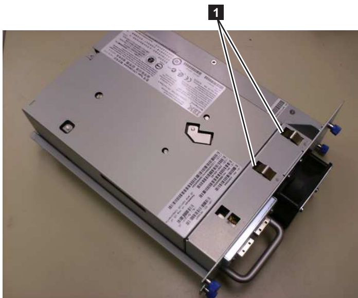
Figure 140. Library drive sled with ESD springs [1] (SAS sled shown)
