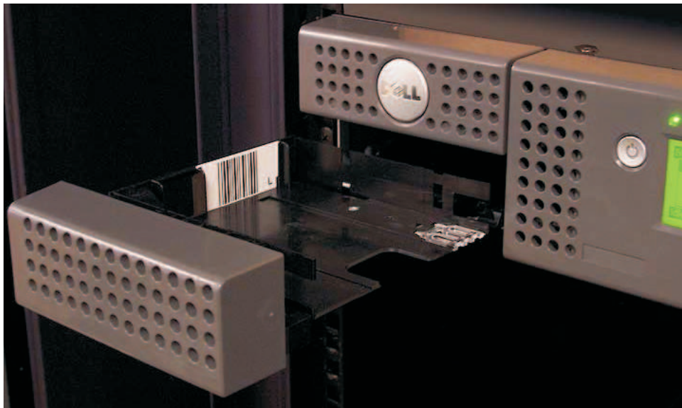
Figure 59. 2U library I/O station in the left magazine
