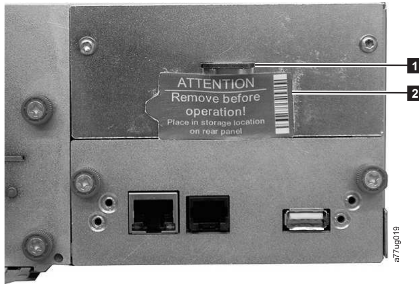
Figure 23. Library shipping lock and label storage location on rear panel of library
