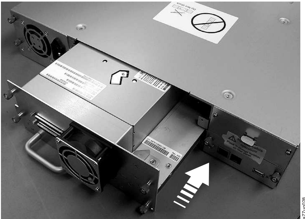
Figure 143. Pushing the drive sled into the library (drive sled without ESD springs shown)
