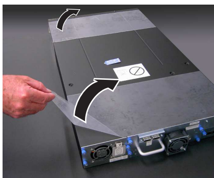
Figure 19. Removing the plastic protective sheets from the library
