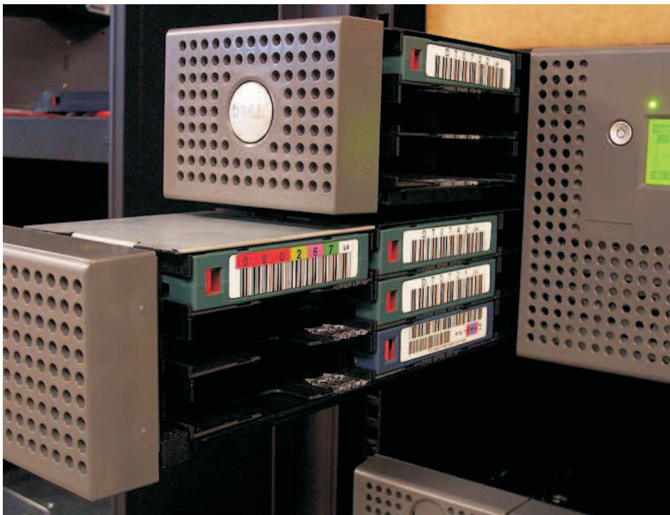
Figure 135. Left Magazines pulled out of the 4U Library
