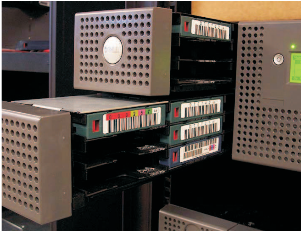
Figure 158. Left magazines pulled out of a 4U library (facing front of library)
