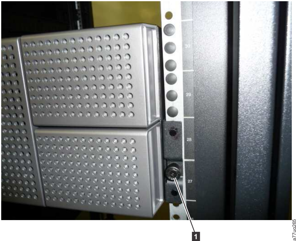
Figure 36. Securing the 4U library to the rack
