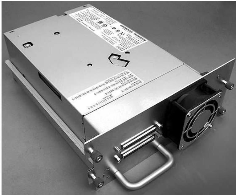
Figure 139. Library drive sled without ElectroStatic Discharge (ESD) springs (SCSI sled shown)
