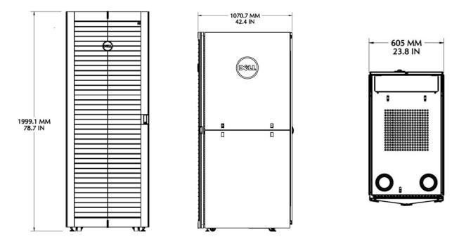
Figure 18. External dimensions – 4220 rack enclosure
