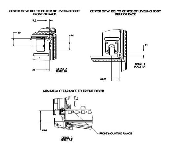
Figure 25. Internal dimensions – 4220D and 4820D (leveling foot/minimum clearance)
