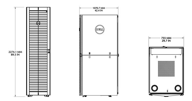
Figure 26. External dimensions – 4820W rack enclosure
