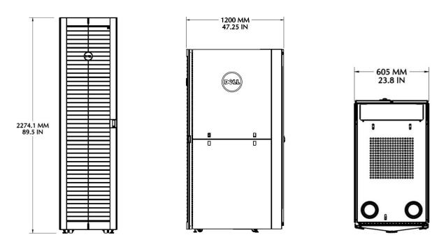
Figure 22. External dimensions – 4820D rack enclosure
