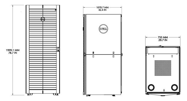
Figure 19. External dimensions – 2420 rack enclosure
