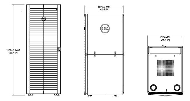
Figure 27. External dimensions – 4220W rack enclosure
