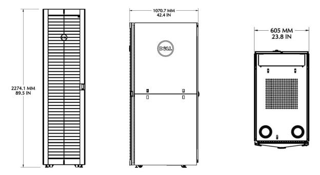
Figure 17. External dimensions – 4820 rack enclosure
