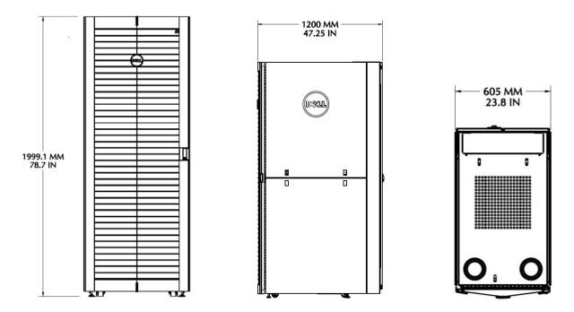
Figure 23. External dimensions – 4220D rack enclosure
