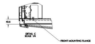
Figure 29. Internal dimensions – 4220W and 4820W (leveling foot/minimum clearance)
