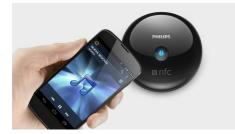
Pair Bluetooth<sup>®</sup> devices easily with one-touch NFC (Near Field Communications) technology. Just tap the NFC enabled smartphone or tablet on the NFC area of a speaker to turn the speaker on, start Bluetooth<sup>®</sup> pairing, and begin streaming music.
