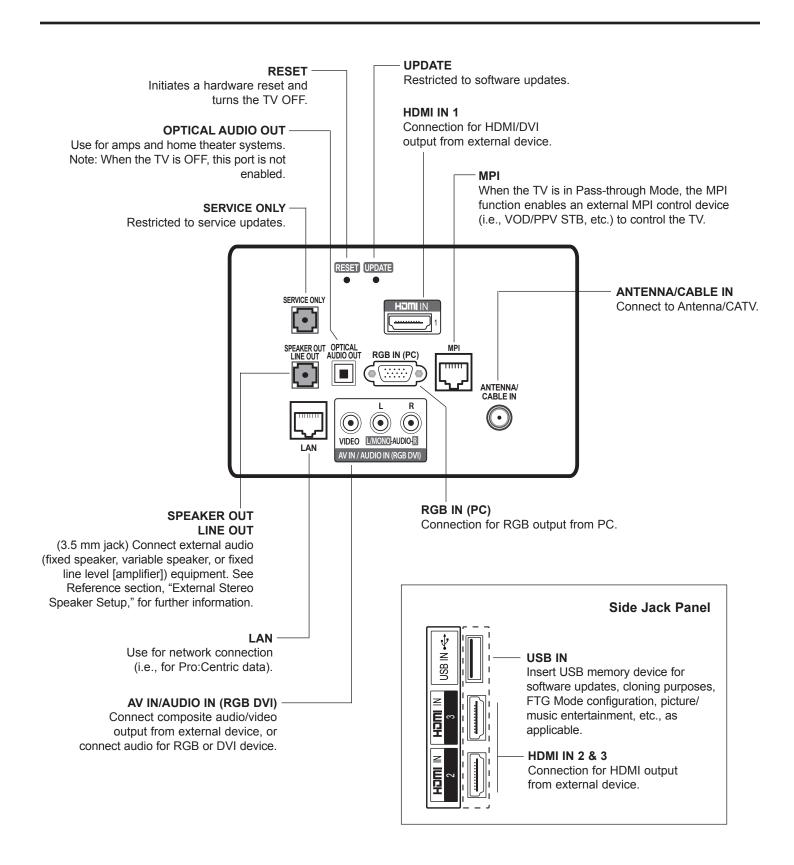
The SPEAKER OUT / LINE OUT 3.5 mm stereo jack on the LX560H rear panel provides stereo speaker signal outputs (fixed speaker, variable speaker, or fixed line level [amplifier]) for external audio equipment. Set Installer Menu item 097 AUDIO OUTPUT as required in accordance with external audio equipment connected to the TV. Also, refer to the following diagram for pinout details.
