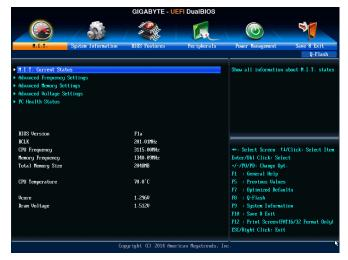
This section provides information on the BIOS version, CPU base clock, CPU frequency, memory frequency, total memory size, CPU temperature, Vcore, and memory voltage, etc.
