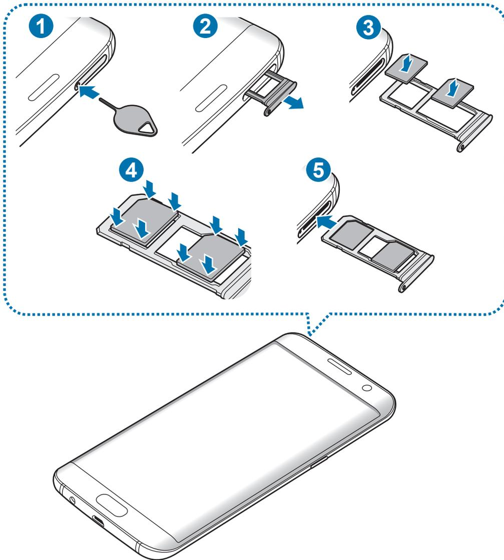
1 Insert the ejection pin into the hole on the tray to loosen the tray.
