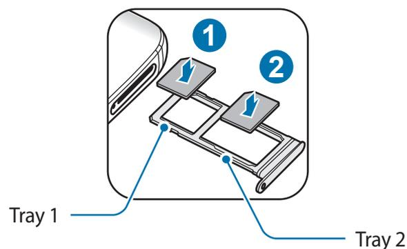
4 Gently press the SIM or USIM card into the tray to secure it.
